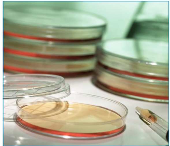
ASTM C1338 determines the ability of new insulation materials and their facings to support fungal growth.
